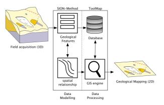
Figure 2 – GIS Framework for digital geological mapping consisting of two components: the SION-Method and TOOLMAP software
