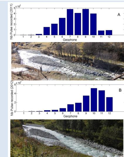
Fig 6 : Riverbed upstream of the section and sum of pulses recorded per geophone for A) 2011 B) 2012
