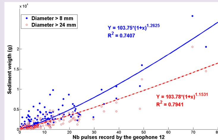
Fig 3 : calibration curve with equation type  $y = a(1+x)^b$  (for plate 12)
