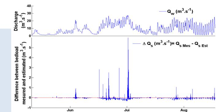
Fig 4 : Year 2012 top, Discharge, bottom, Difference between estimated (Recking in press) and mesured bedload
