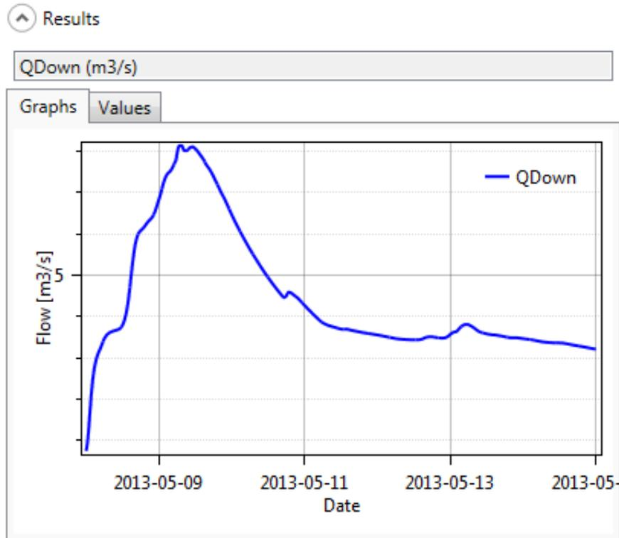
**Figure 97** Hydrograph in the outlet of the system
