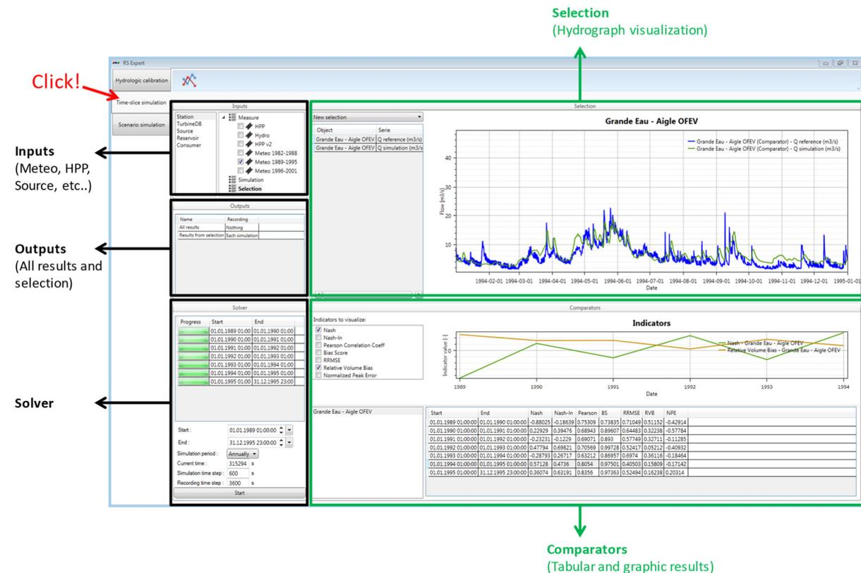
**Figure 68** Interface of the Time-slice simulation tool (in black: configuration; in green: results)
