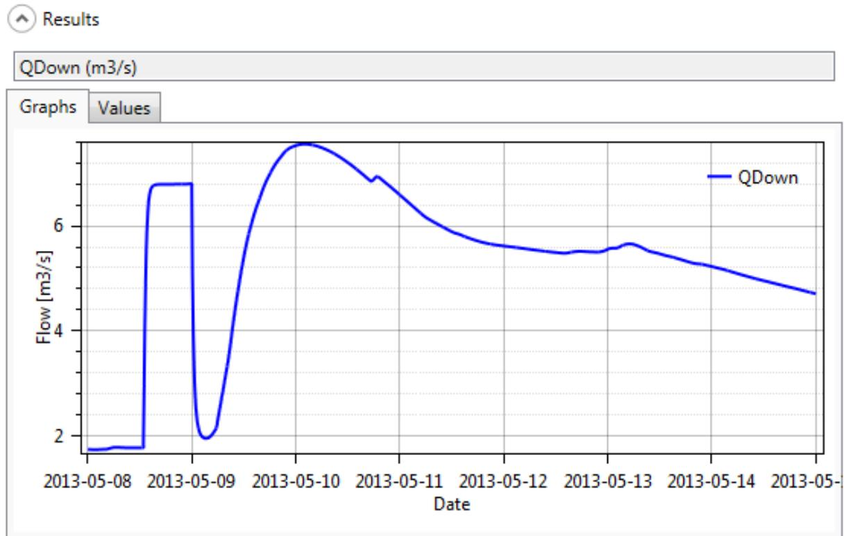
**Figure 116** Outlet hydrograph after the addition of the new release. Peak discharge of  $7.552 \text{ m}^3/\text{s}$  arrives now on May the 10<sup>th</sup>, 2013 at 02:10.
