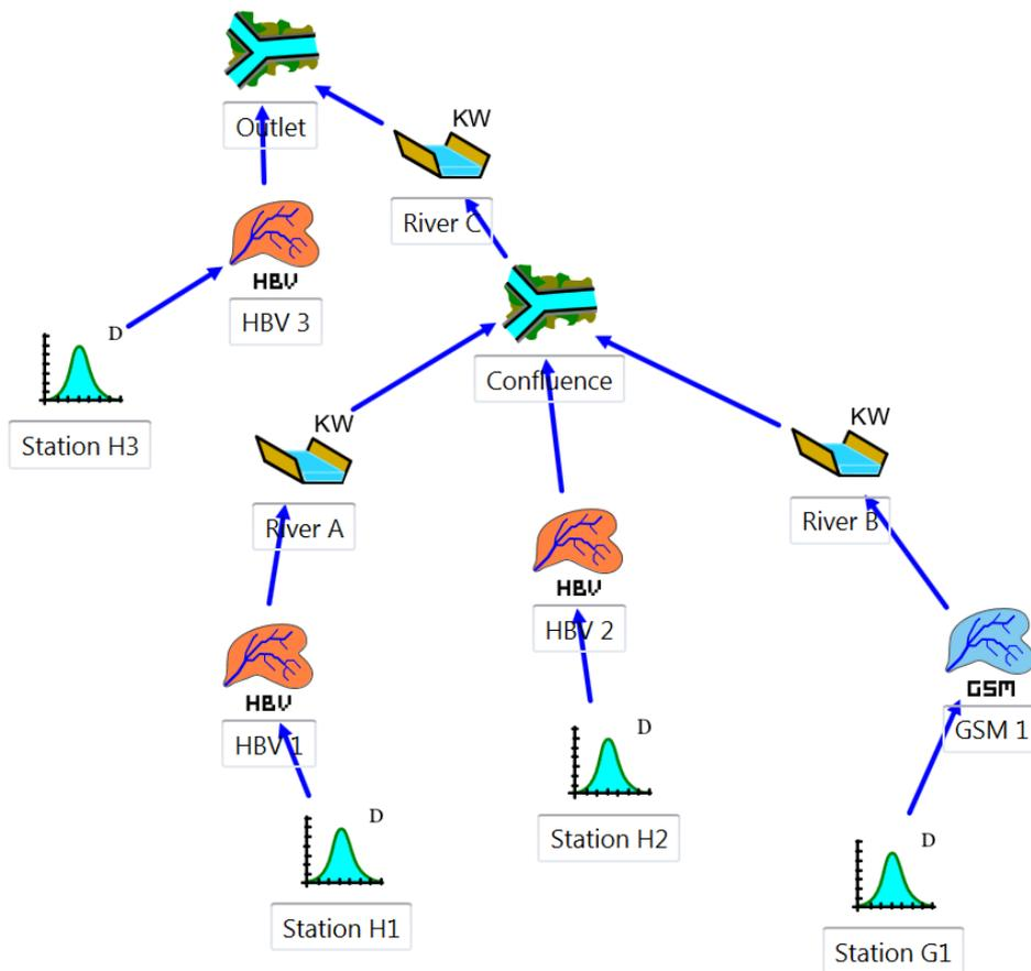
Figure 90 Topology of the full model: production, transfer then transport
