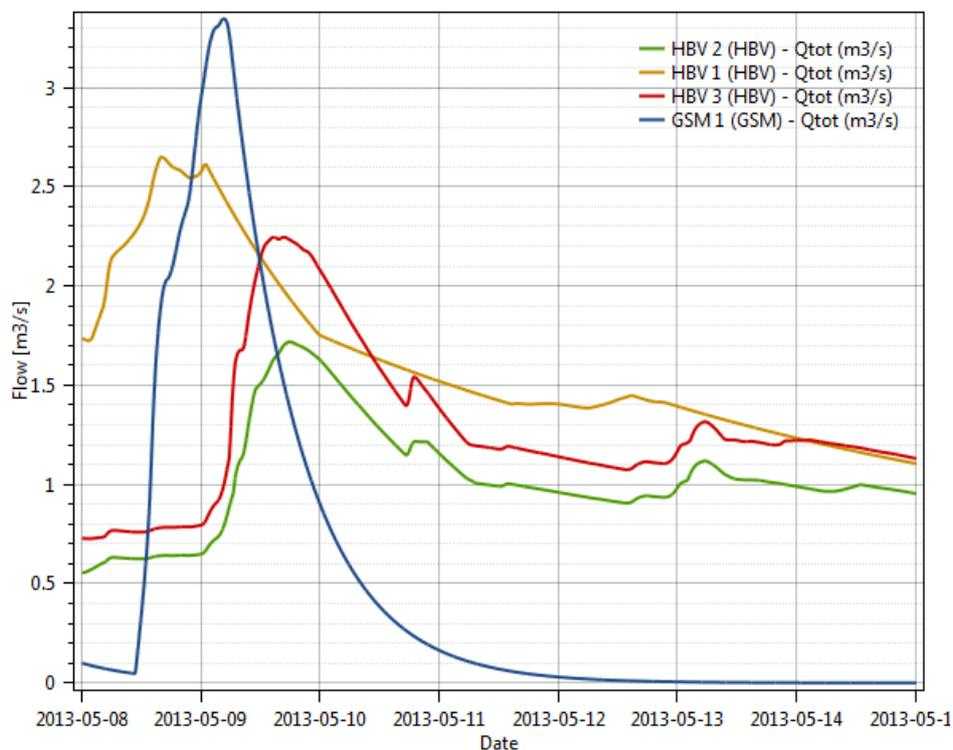
Figure 100 Hydrographs at the outlet for each sub-basin of the system
