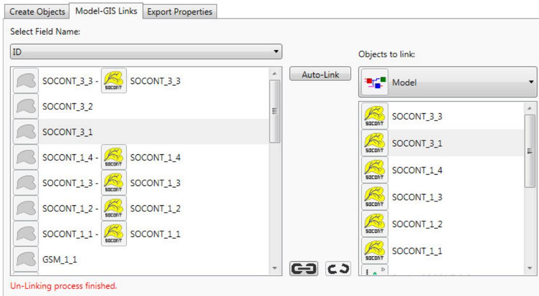
**Figure 49** Linking and unlinking elements. Here, the two unlinked elements are ready to be linked.
