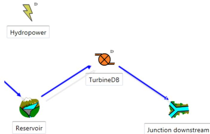
**Figure 20** Addition of a *Hydropower* object
