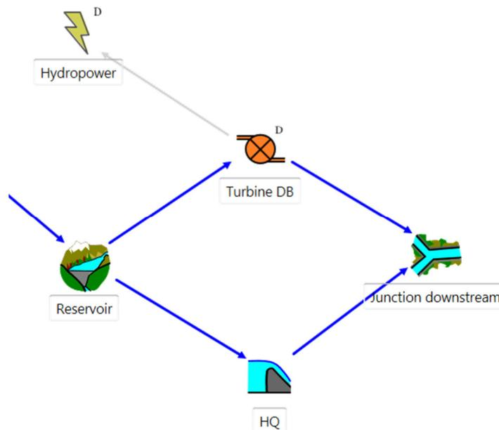
**Figure 22** Addition of a spillway
