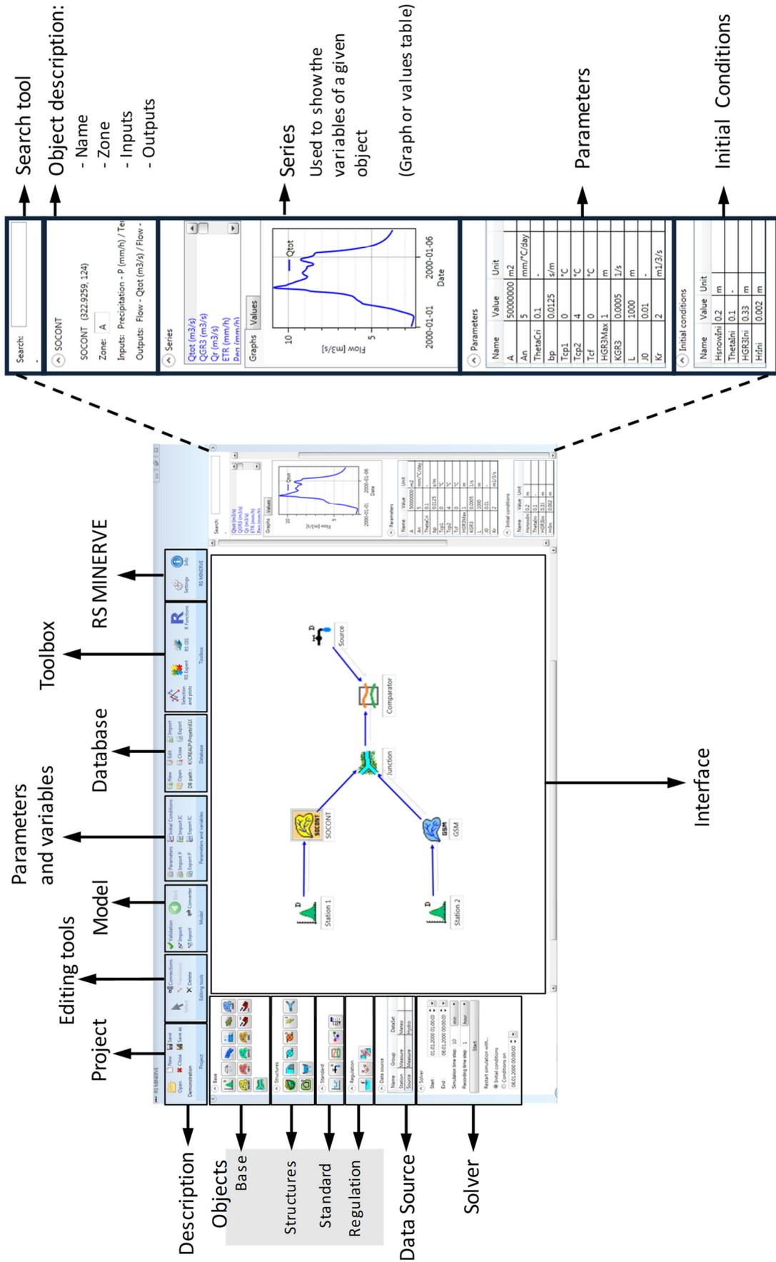
Figure 1 Structure of the RS MINERVE main interface
