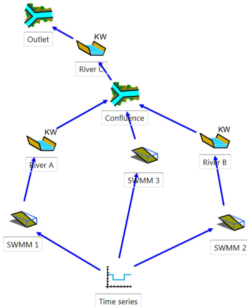
**Figure 76** Topologic links between the different objects from the model
