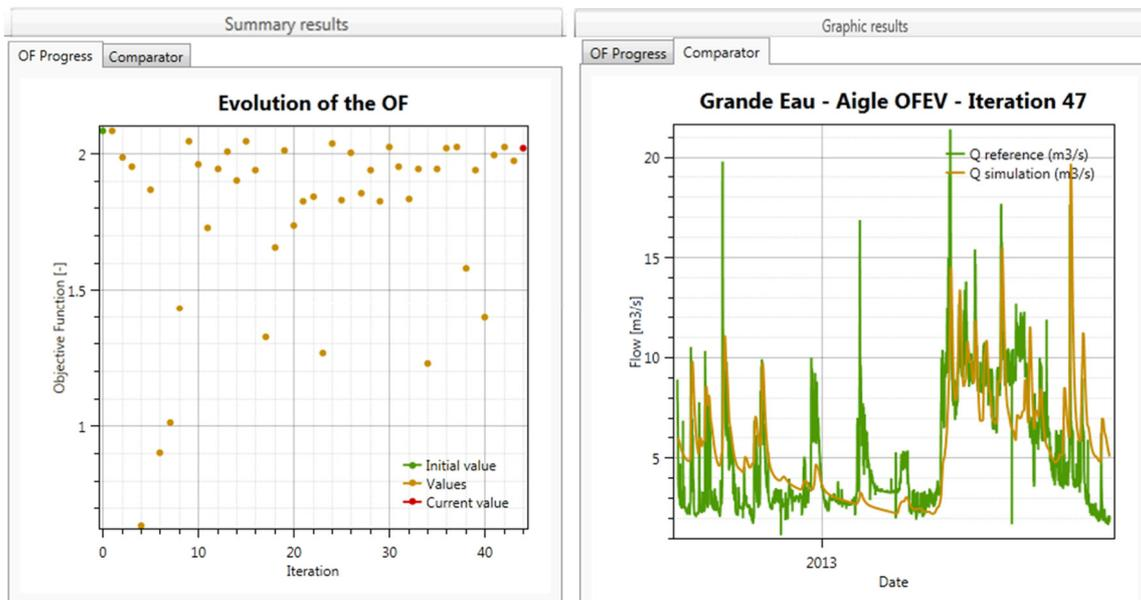
**Figure 58** Graphic results of the calibration in progress. Evolution of the Objective function (left) and hydrograph of both observed and current simulated discharge (right).
