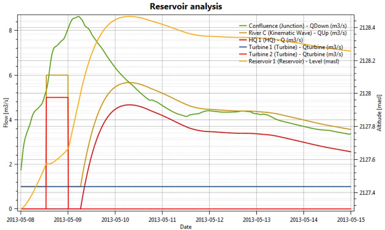
**Figure 117** Flows balance of the reservoir and hydrographs at main control points
