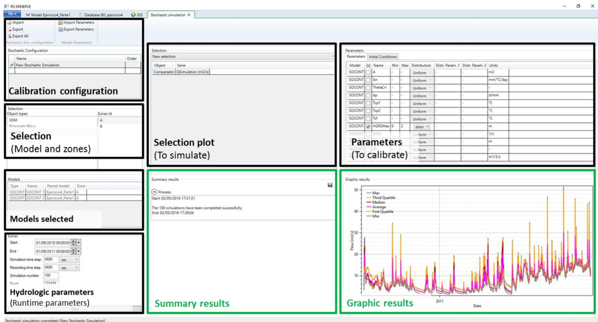
**Figure 63.** Interface of the Stochastic simulation module (in black: configuration; in green: results)
