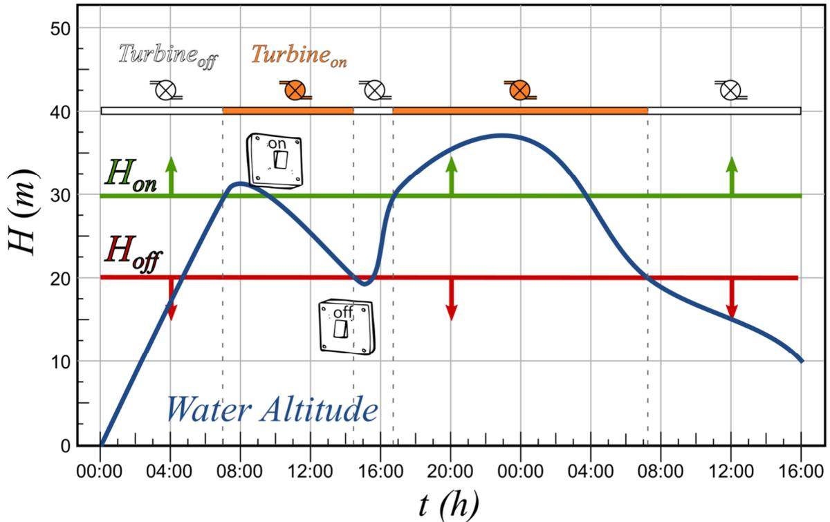
Figure 19 Example of turbine operation
