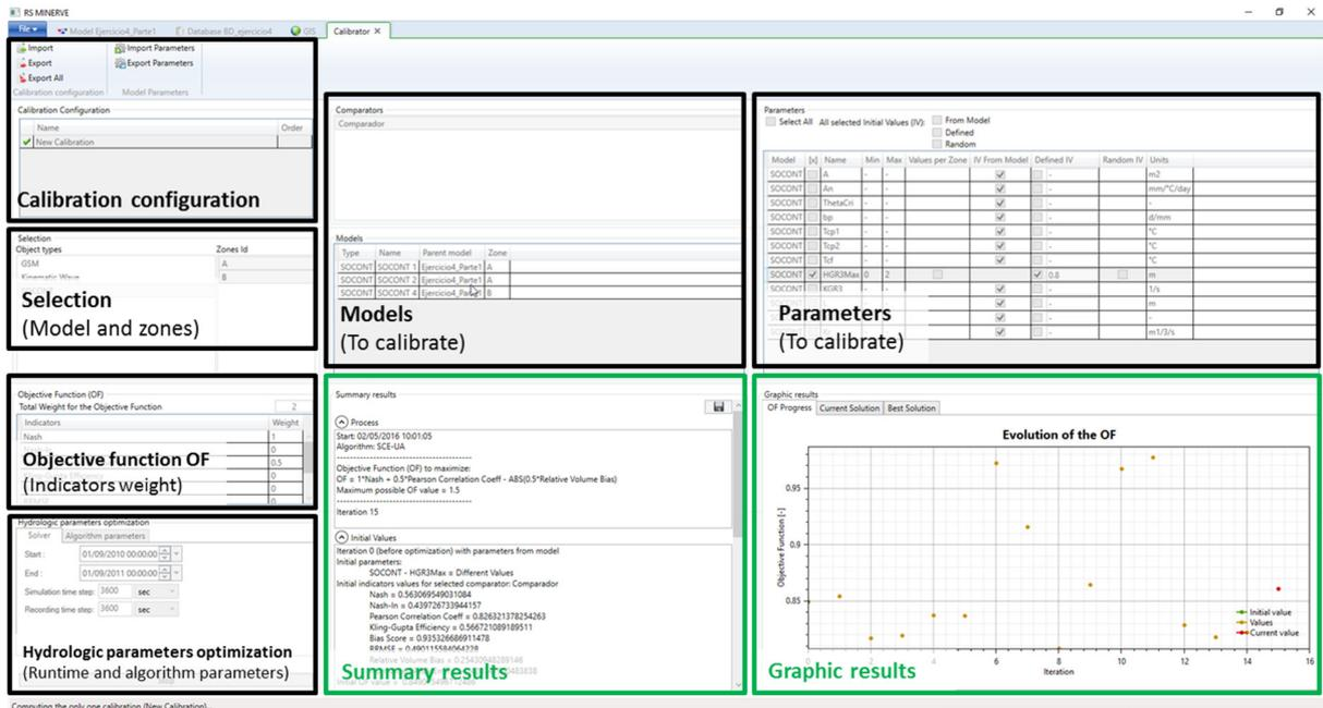
Figure 55 Interface of the Hydrological calibration module (in black: configuration; in green: results)
