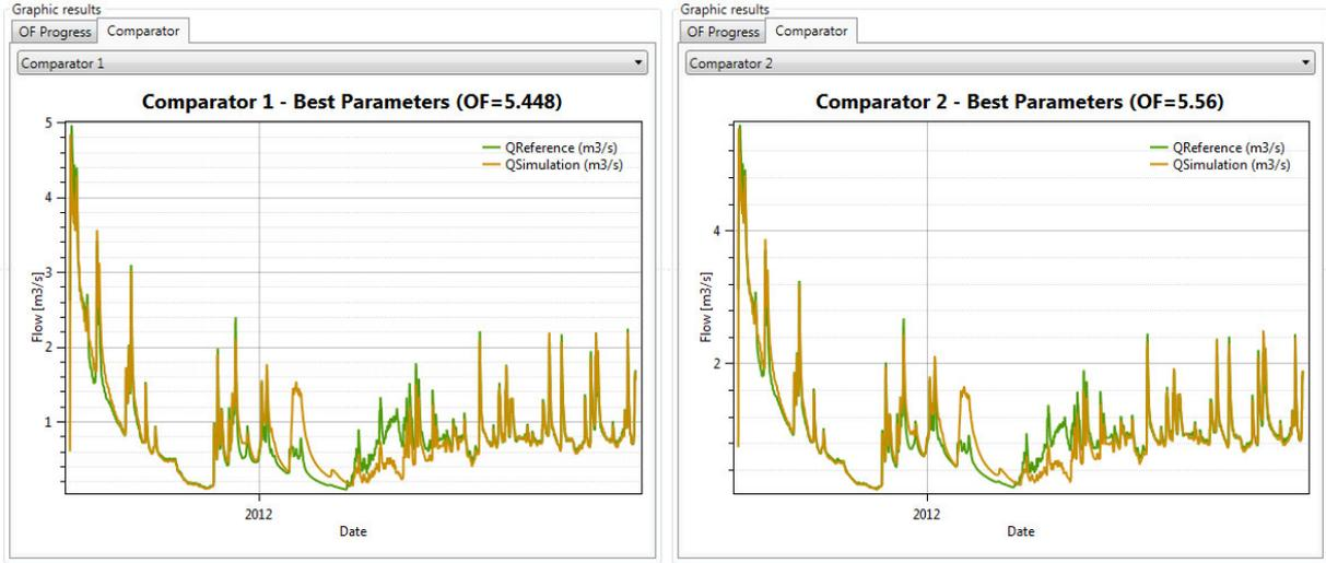
**Figure 133** Graphic results of the calibration. Hydrograph of both observed and current simulated discharge
