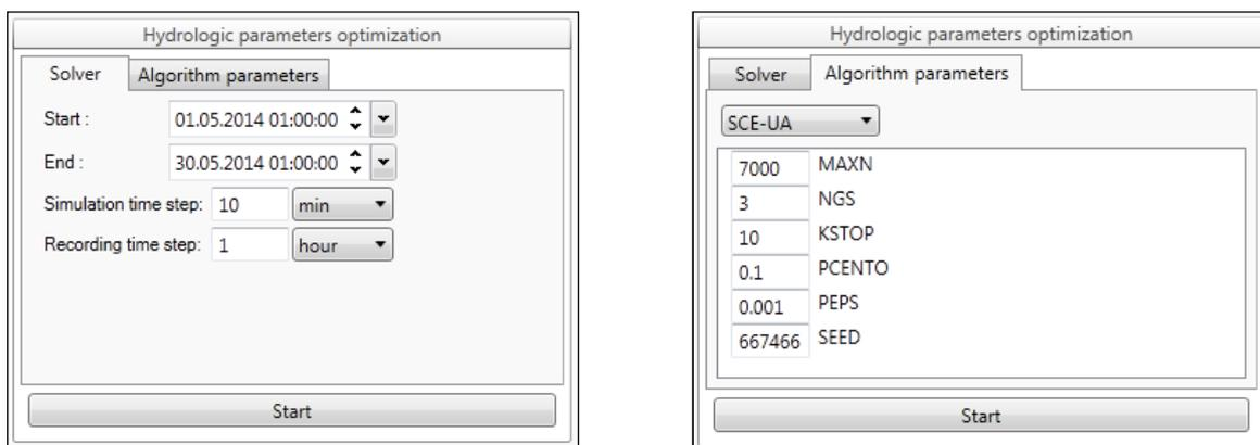
Figure 56 Calibration solver: both runtime (left) and algorithm properties (right)
