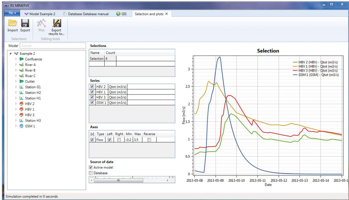
Figure 99 Selection and Plots with the hydrographs at the outlet for each sub-basin of the system
