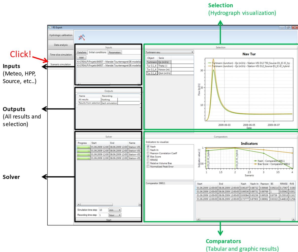
Figure 60 Interface of the Scenario simulation module (in black: configuration; in green: results)
