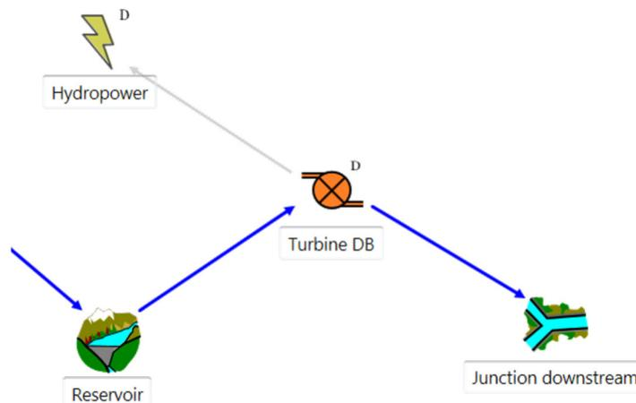
**Figure 21** Links between the *Hydropower* object and the *Reservoir* and *TurbineDB* information
